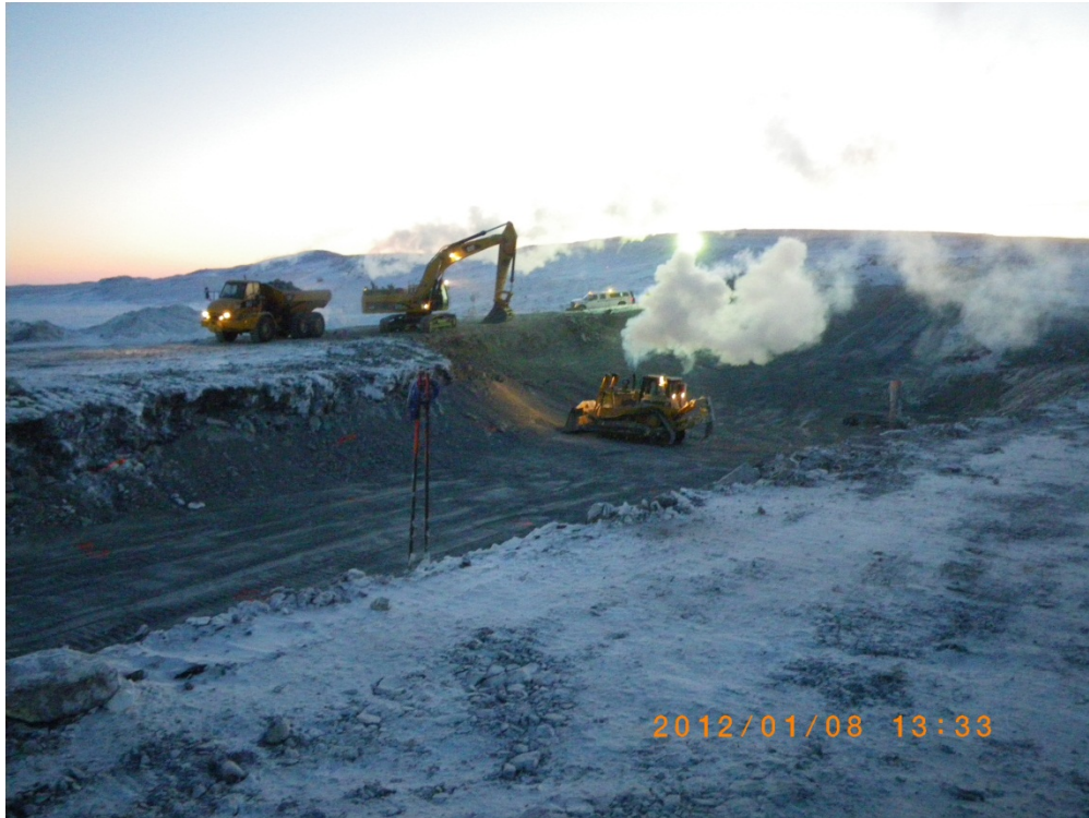
Photo 2: The dozer pushing the 5/8" clear material to the excavator with then mixes it with ROQ when loading the haul truck.
